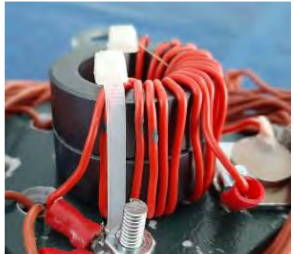
49:1 showing 2xFT140-43 ferrite cores. No case, insulated wire protects windings from moisture.
