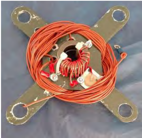
49:1 transformer on winder. Note the silicone coated ultra flexible wire and SO-239 jack
