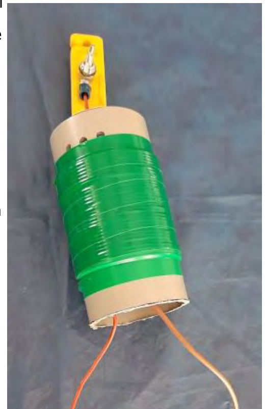
35 microhenry loading coil for 40m band. Note the 20m drop wire and 40m tail wire.
