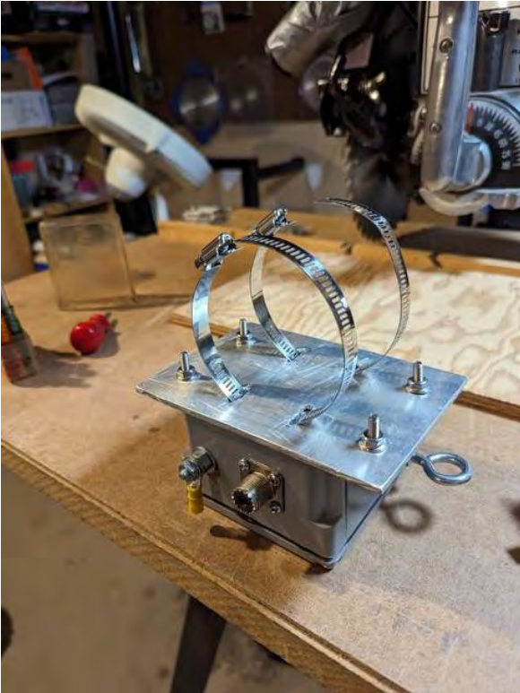
Attachment for the UNUN to the stack - aluminum plate and pipe clamps. Rubber shims were used at the plate-to-mast interface.
